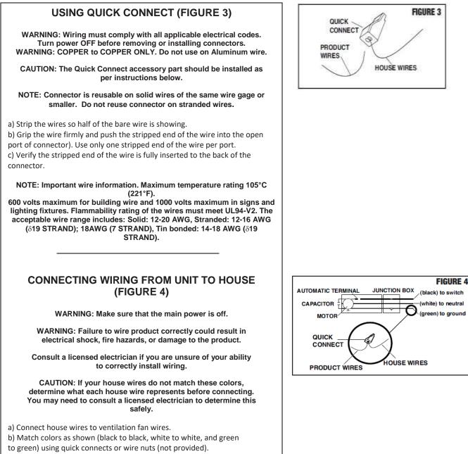
c) Replace the junction box cover. Do not pinch the lead wires
