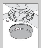
Lift the globe and align the notches in the globe with the tabs in the light kit. Attach the glass bowl to the light kit by twisting it clockwise until it snaps into place.
