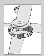
Install a bulb into each of the sockets. When necessary, replace with bulbs of the same type and wattage.
