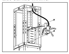
Remove wiring cover and connect house wiring to hood wiring – black to black, white to white, green to green. Reattach wiring cover.
