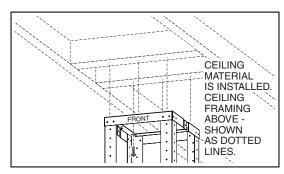
After ceiling surface is finished, align frame assembly to ceiling framing, and attach to ceiling framing with (6) 4mm x 38mm screws. Tighten securely, making sure that the upper frame bracket is tight against the ceiling.
