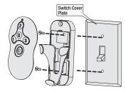
To install the transmitter cradle, remove the two screws holding the switch cover plate. Do not remove the cover plate. Orient the cradle by lining up the two mounting holes with those on the cover plate. Insert and tighten the screws. Do not over tighten.
