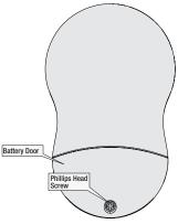
To access the battery compartment, remove the small Phillips head screw that secures the battery door to the transmitter assembly. The battery should be installed with the positive (+) side up. Replace with a CR2032 battery when necessary.
