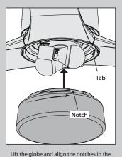
Lift the globe and align the notches in the globe with the tabs in the light kit. Attach the globe by lifting and twisting clockwise until it rests firmly in place. Congratulations! YOU'RE DONE! See next page for remote operation instructions.
