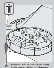
hardware bag halfway into the motor housing. It does not matter which two screw holes you choose.
