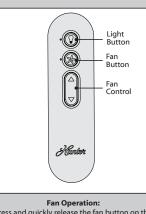
Press and quickly release the fan button on the remote control to turn the fan OFF or ON. Use the fan control directional pad to raise or lower the fan to the desired speed. Press and hold the fan button to reverse the fan direction.
